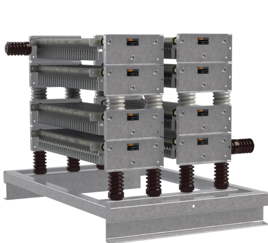
IP00 resistor: 14 Ohm. 500 Amp. -10 sec Insulation level: 12 kV.
